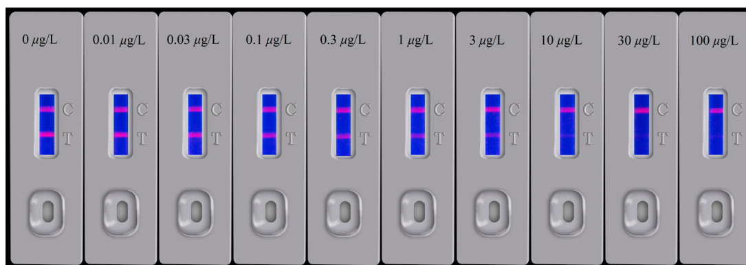
Figure 3. Series of diluted derivative solutions tested by fluorescent ITSA for nitrophenylAOZ in buffer and visual results examined after 10 min. Concentrations are expressed as equivalent underivatized AOZ. Sample was spiked with AOZ at levels of 0, 0.01, 0.03, 0.1, 0.3, 1, 3, 10, 30, and 100 \mu\text{g/L} .
